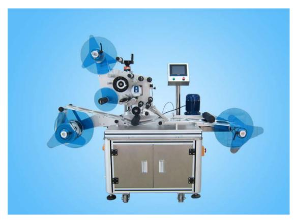
This converting machine has the functions of single converting only, can be used for various specifications of material object converting, such as cloth roll, paper roll, label roll, equipped with flat converting function; Can be equipped with color tape printing machine, inkjet code machine, label and print production batch number and other information.
